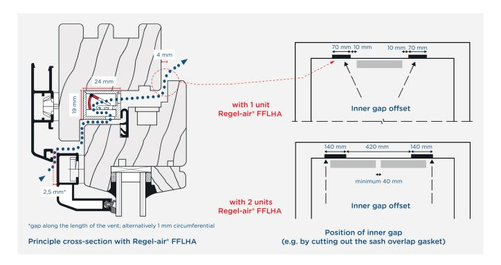
The Regel-air® window rebate vent FFLHA Type 24 FL is generally installed in the top of the window frame or transom. Type 24 RF is suitable for vertical installation (see back). The vent is 24 mm deep, 19 mm high and 290 mm wide.
